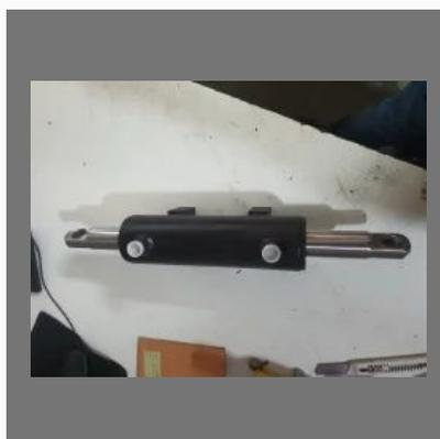
GX300D Forklift Power Steering Cylinder
